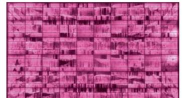
An electroluminescence test showing numerous cell fractures in a solar module
