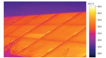
Thermal imaging uncovering defects in solar modules
