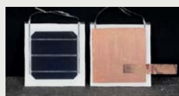
Figure 12: Bonding of the one-cell-mini modules with adhesive copper foil during the PID test, unprepared sample (left) and prepared sample (right).
